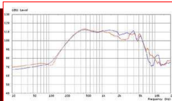
▲ Mid response with phase bung (blue) & without (red)
