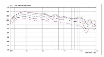
0/10/20/30/40/50 degree off-axis horizontal HF response (wide-axis).
