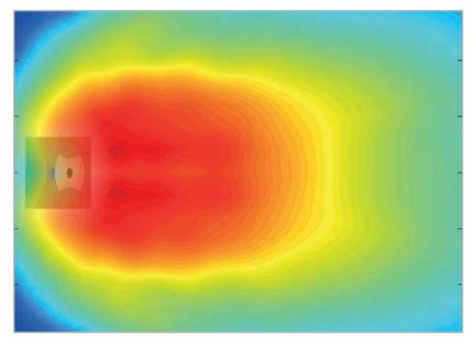
• XE500 SPL @ 6.3kHz over a 3 x 4m plane at head height Each contour represents 0.2dB change; yellow is -6dB
